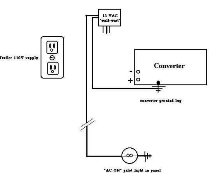
Simple work-around to keep the pilot light function when phasing out the "Univolt" per Bill Worden
